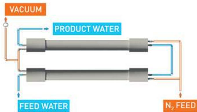
Figure 3. Membrane deaeration system in "Combo" mode
