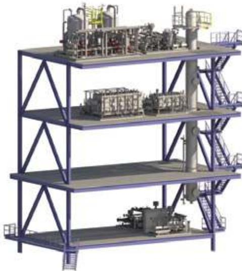
Figure 6. 3D Model of Vacuum Tower system
